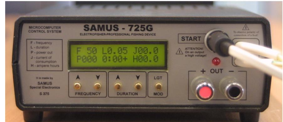
Sockets "OUT ( see photo) serve to install a loading of electrofisher. The socket "+" is connected with cable on the landing net. The socket "-" is connected with outer cable with metal wire at the end (mass/minus) which is thrown into water behind the boat or fisherman.
