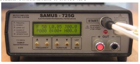
Sockets "OUT ( see photo) serve to install a loading of electrofisher. The socket "+" is connected with cable on the landing net. The socket "-" is connected with outer cable with metal wire at the end (mass/minus) which is thrown into water behind the boat or fisherman.
